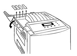
2 Open the plastic bags and take out the toner cartridges. Shake the toner cartridges several times.
